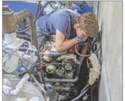
A Mariner Scout Ship 'Tradewind' crew member working on the generator's cooling system.
