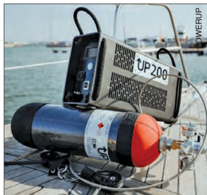
Clockwise from top left: Ivar Krusenbergs looks over his company's 1,000-watt hydrogen fuel-cell generator on board 'Gerda' earlier this year; Sean Shigley, right, and Cree Partridge were all smiles for 'Gerda's' seatrial; a smaller version of PowerUp's hydrogen-powered generator.
