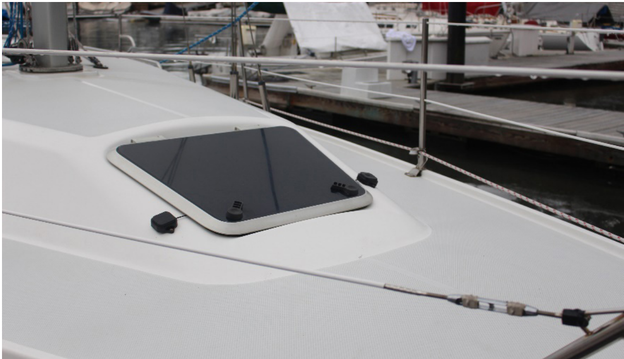
Figure 3. Dual antennas on the foredeck of the Pacific Spirit
