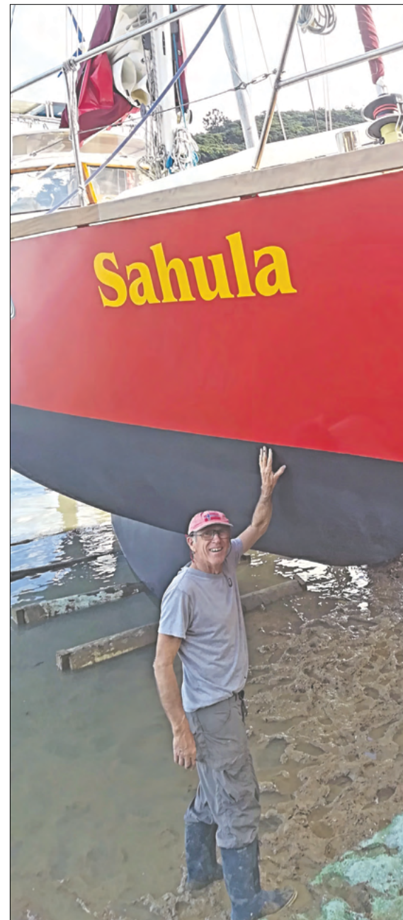
David inspects 'Sahula' at Mickey Mouse Marine, a tidal grid yard near Lin's home on Kawau Island. ('Tidal grid' means you pull in, tie off, and wait for the tide to go out. No Travelift required!) Right: The boat underway.
