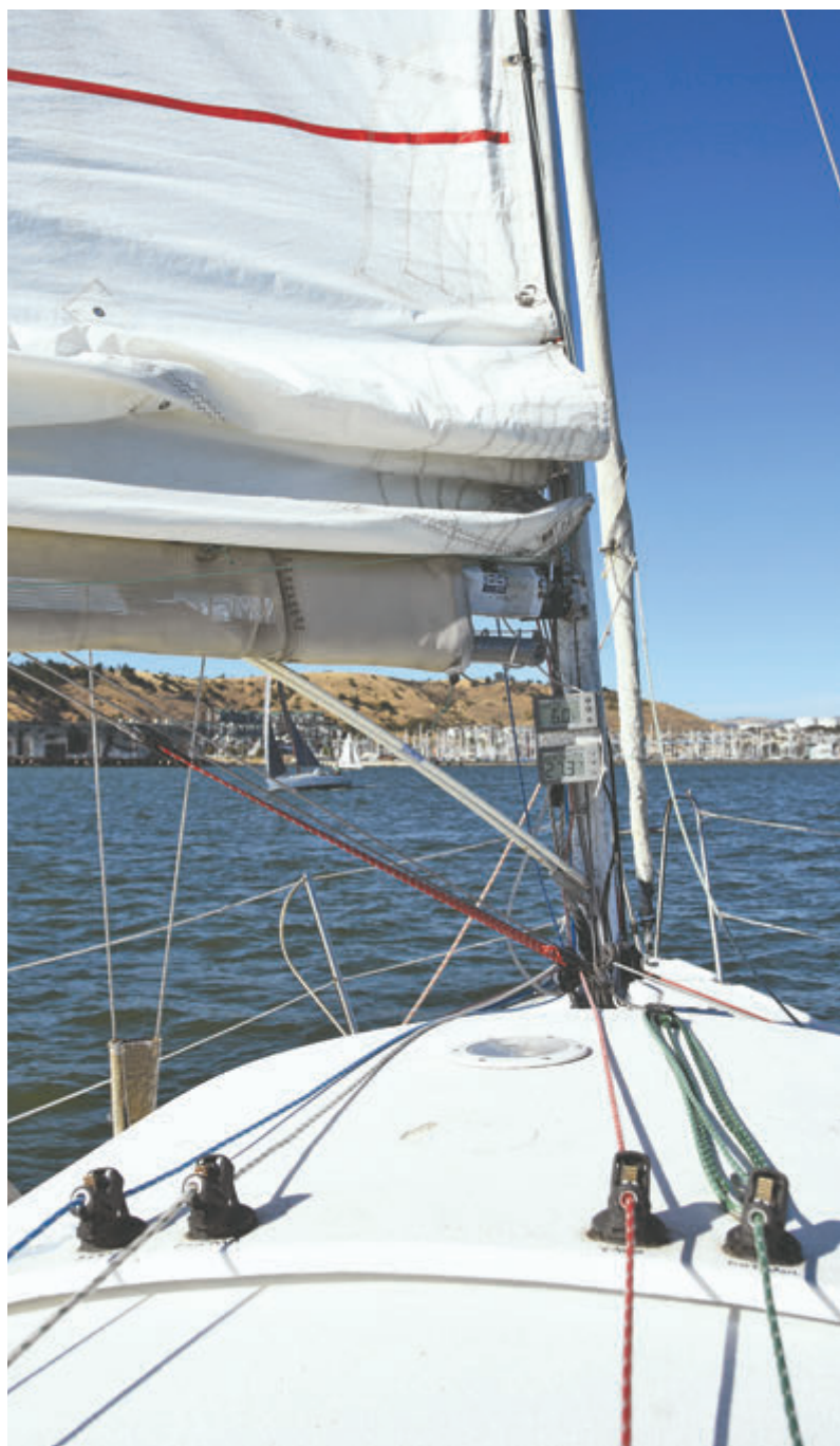
A bunch of fiddly lines. Left, from left to right: Reef 1 tack, cunningham, boom vang, outhaul. Above: Spinnaker halyard, spare jib halyard, reef 2. Below: Reef 1 clew, primary jib halyard, the two-to-one main halyard. The lazy jacks are easier to see in the photo on the opposite page. Not shown: backstay, traveler, jib furler, spinnaker twings, topping lift, downhaul.
