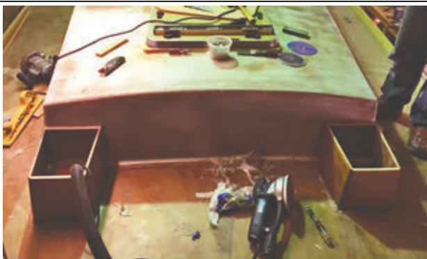
Talking shop. Below: Framing up bases for the dodger and hatch. Below left: Interior finish work has begun. Center left: Garth's design looks both pretty and practical. Above left: Garth in the shop. Above: The dorades go in.
