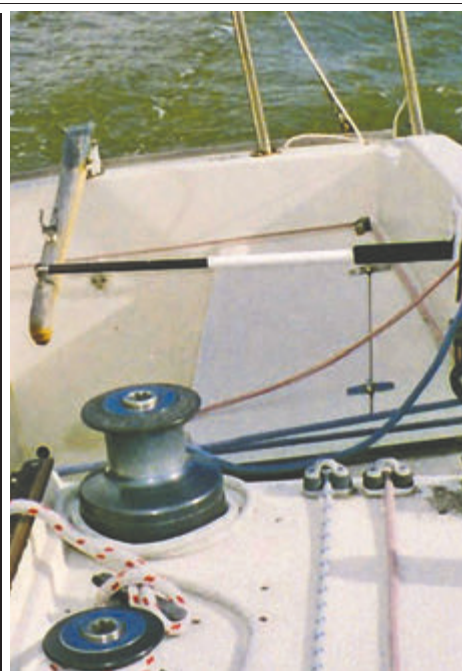
Above left: Not all designers get this right. Some rudders have the notch way too high. Center: This rudder notch is too low. It's not very useful for climbing aboard, and bad hydrodynamics. Right: The best tiller-locking system. Don't skimp; get one for each side.
