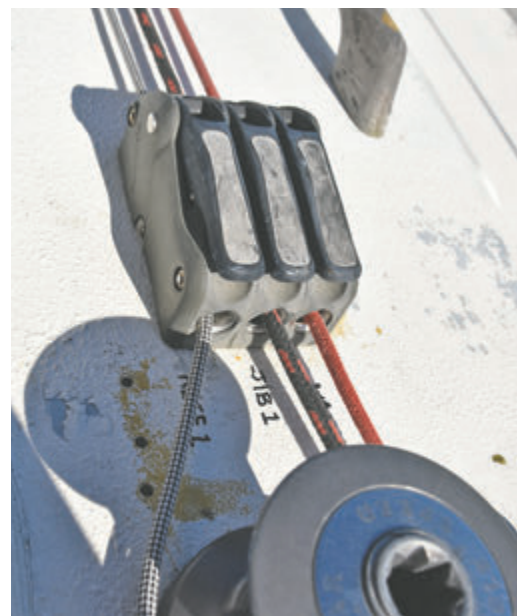
A bunch of fiddly lines. Left, from left to right: Reef 1 tack, cunningham, boom vang, outhaul. Above: Spinnaker halyard, spare jib halyard, reef 2. Below: Reef 1 clew, primary jib halyard, the two-to-one main halyard. The lazy jacks are easier to see in the photo on the opposite page. Not shown: backstay, traveler, jib furler, spinnaker twings, topping lift, downhaul.
