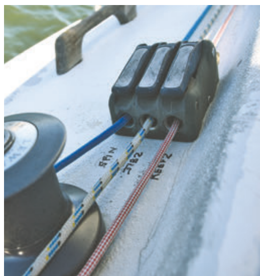
A bunch of fiddly lines. Left, from left to right: Reef 1 tack, cunningham, boom vang, outhaul. Above: Spinnaker halyard, spare jib halyard, reef 2. Below: Reef 1 clew, primary jib halyard, the two-to-one main halyard. The lazy jacks are easier to see in the photo on the opposite page. Not shown: backstay, traveler, jib furler, spinnaker twings, topping lift, downhaul.
