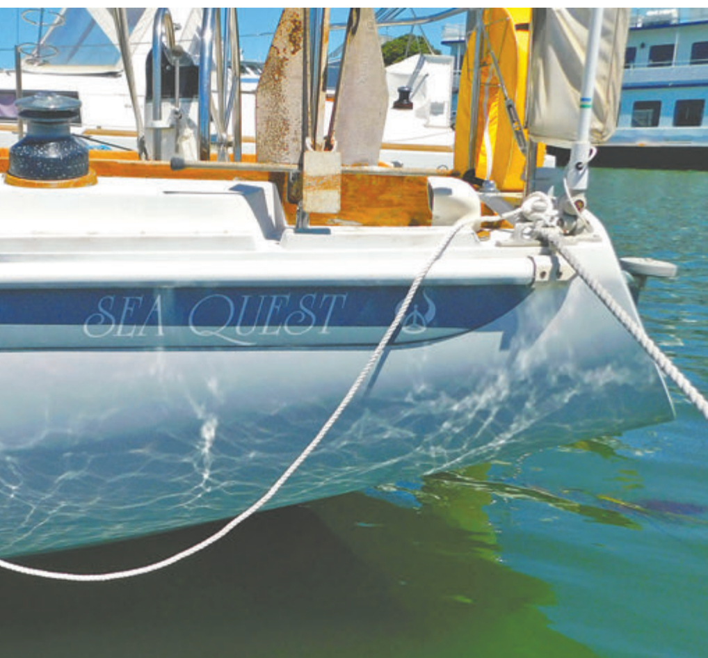
Dockline rigged as an emergency one-step boarding ladder. The step height should be about at the waterline when in use.
