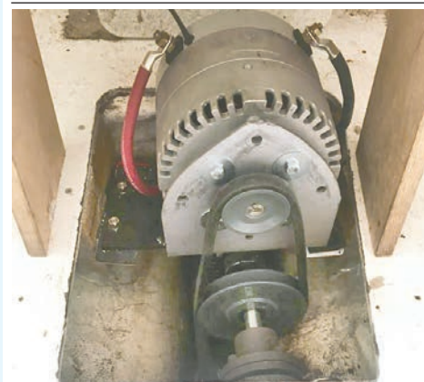
The hope was that the motor might fit out of sight below deck, but in the end it ended up in this higher position, with a belt driving the shaft.
