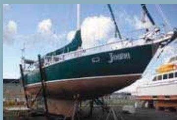
Coppercoat applied 2008, now 12 years old
