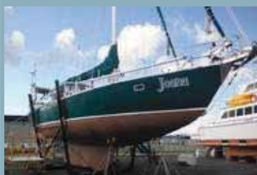
Coppercoat applied 2008, now 12 years old
