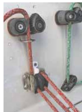
A simple spacer to prevent traveler lines from getting fouled.
