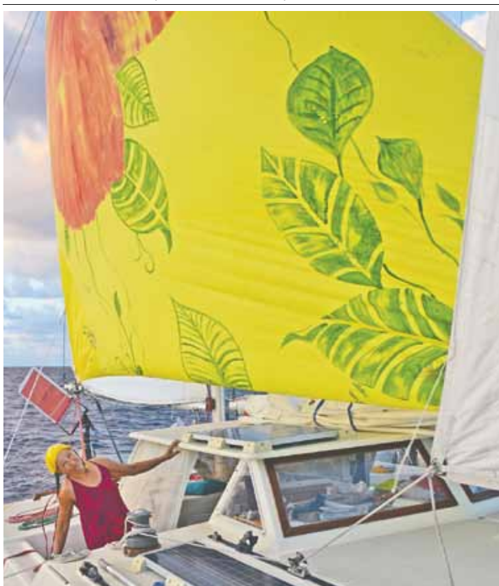
One cool thing about a ketch rig is if you're unable to use your mainsail or mainmast for whatever reason, you can fill that slot with a mizzen staysail. Ours was put to good use during the long slog to Nuku Hiva.
