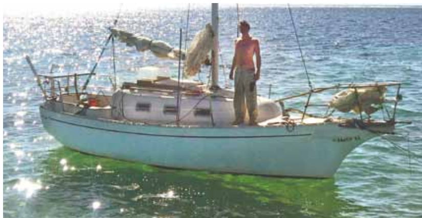
'Tish' at anchor. Not often seen in far-flung cruising grounds, the jaunty little Bayfield 25s are '70s-built Canadian pocket cruisers featuring shoal draft (3 feet) full keels and 6 feet of interior headroom.
