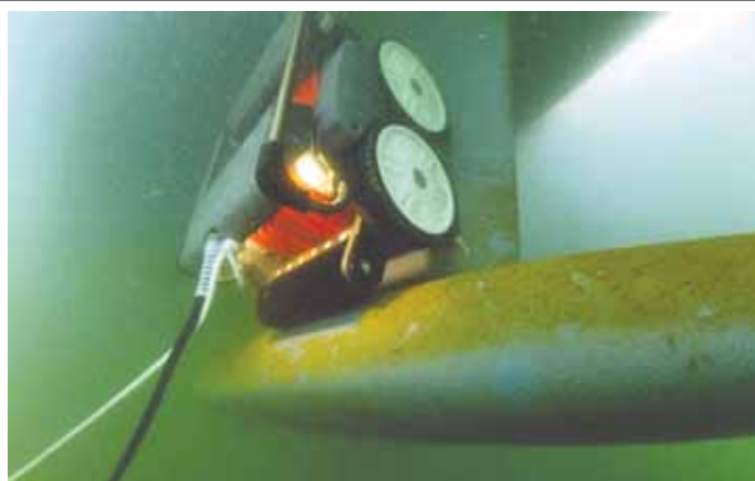
The Keelcrab (left) and the Hulltime drones can clean your bottom, but they still need a human driver to steer while watching the video feed.
