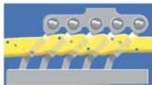
**✓** ...Lewmar's Domino mechanism flexes it for better grip and less rope wear. Dominos also allow multiple holding points.
