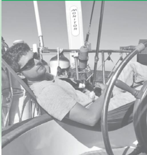
“The biggest boon has been the Monitor self-steering windvane. I can’t say enough about this ingenious framework of stainless steel. Not only does it draw zero energy, deriving all of its power from the wind and leverage from mechanical gears, it steers the boat flawlessly and efficiently. It steers the boat 98% of the time.”
