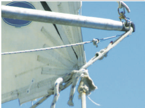
A small sacrificial pennant turned out to be the perfect solution for wear and tear on the clew of the genoa.
