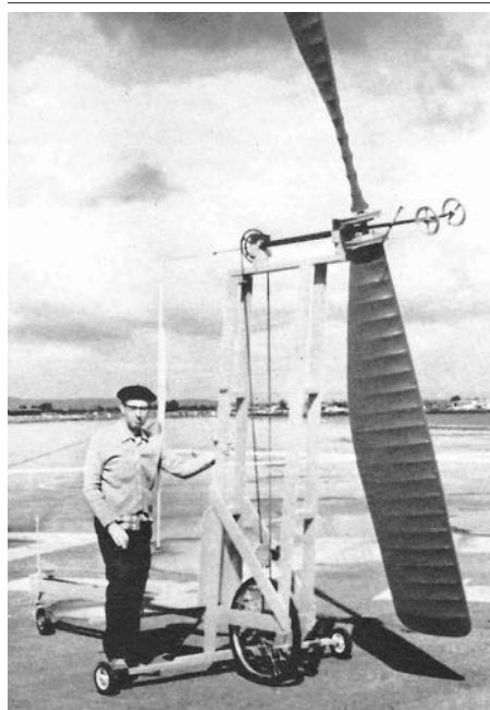
Sir Isaac Helm prepares baby Lee's stroller for an outing, circa 1975. (But seriously, this 'land yacht' of the mid-'70s was able to achieve downwind speed in excess of true wind speed.)
