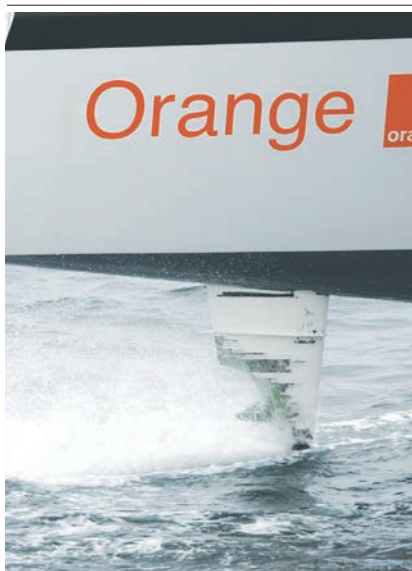
Spread, the perfect storm rider, Bruno Peyron's mighty 'Orange II'. Above, the broken port rudder continued to delaminate — and disintegrate — the whole way across.
