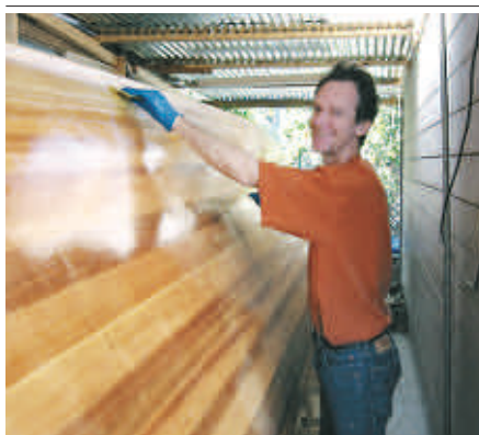
Shown here in the final stages of glassing, Glenn's new boat was built to an ancient design using modern materials. Still no engine!
