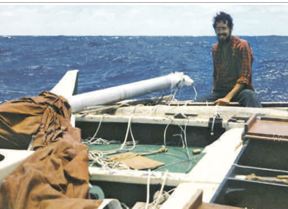
Glenn's crewman Bernard prepares to re-step 'Peregrine's' mast after a shroud broke, dismasting her 1,000 miles from land.
