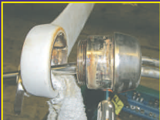
Seven-year-old spreader tip corrosion on a 52-ft racer/cruiser
