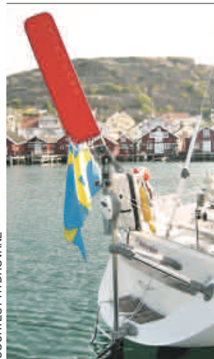
Hydrovanes have been used successfully as emergency rudders.
