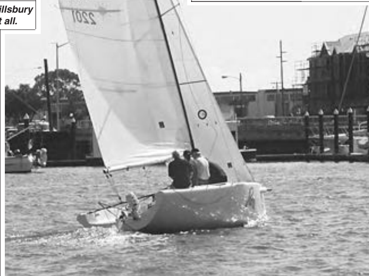
The slick little Rocket 22 is a new incarnation of a Gary Mull design, which now features a retractable bulb keel for easy trailering.
