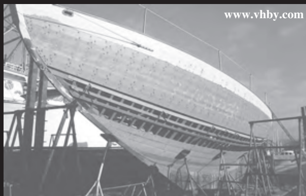
Cherrio II, 46' yawl, complete hull replacement
