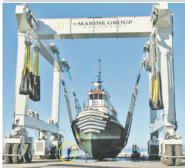
Marine Group's new Travelift hardly breaks a sweat lifting this harbor tug. Note the size of the guy (circled) powerwashing the bottom.
