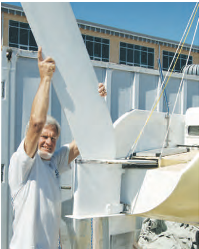
Left to right: Like the rudder on a sailing dink, Gordie's new rudder blade slides out when not in use; the center console keeps the deck clear and lines running smoothly; the slide out ice box will make it easy to grab a cool one.
