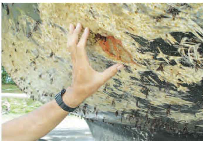
Launched in 1981, you'd think that 'Whinchat's hull was purpose built for reef bashing. Her hull is nearly an inch thick.
