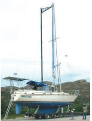
Hauled from the water by one of Marina Seca's purpose-built trailers, this sailboat gets its mast pulled by a special crane before it heads north.
