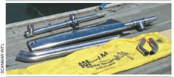
This emergency rudder breaks down into several parts which are easily stowed, taking up minimal space.
