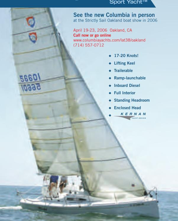
LOA: 30'0" - LWL: 27'0" - Beam: 9'6" - Draft (keel up): 2'8" - Draft (keel down): 7'0" - DISPL: 3995# - Ballast: 1400# SA (Main and Jib Triangles): 433 ft² - SA (Class Spinnaker): 918 ft² - SA/D: 27.96 - Maximum SA (Downwind): 1486 ft² - DISP/L: 88.46 - Headroom (Main Salon): 5'10"
