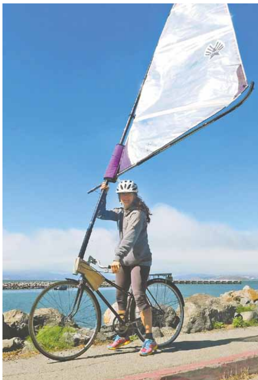
Lee's version, based on an old three-speed bike, rigged with the high-wind sail. The rig is made entirely from discarded windsurfer parts. The pedal-powered drive train is left in place, handy for getting out of irons.
