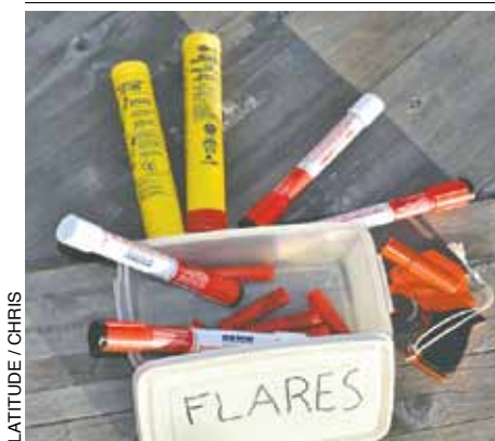
A collection of flares off a Bay Area racer/cruiser. Some are current, some expired.
