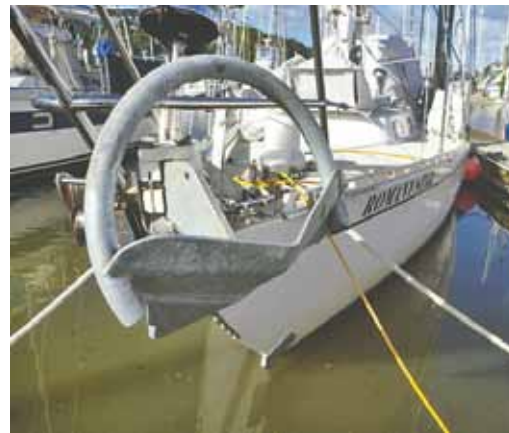
Damage to 'Romany Star's bow included a mashed toe rail, mangled bow roller/chainplate and ruined anchor — but the latter saved the day.
