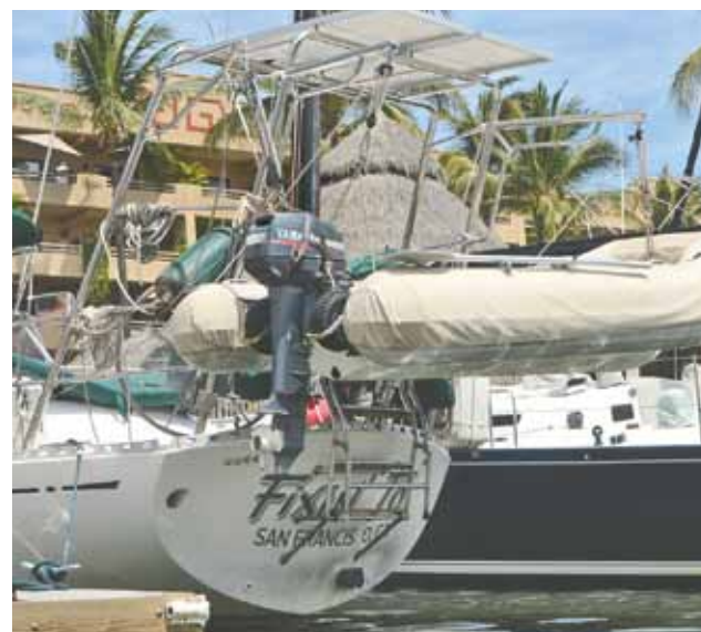
Variation on a theme: This arch is much taller, so crew can access the transom-mounted swim ladder. As with similar designs, the solar panel on top gets full sun all day.
