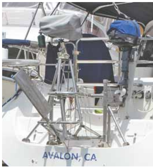
This Monitor windvane has piloted 'C'est la Vie' safely for thousands of miles of Pacific voyaging. The stainless steel rudder swings up (left) when not in use.
