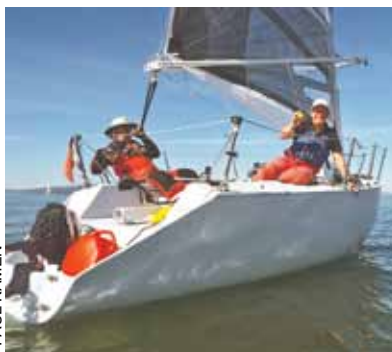
'Critical Mass', the heavily modified Mancebo 24, sports a wishbone boom.
