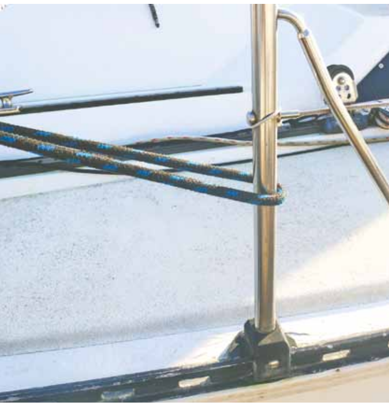
A quick way to estimate friction coefficient between sheet and steel, without moving from the windward rail: Wrap a sheet a half turn around a stanchion, pull at right angles to the stanchion, then angle slightly up or down. The tangent of the angle at which the bight of rope starts to slip is the friction coefficient.
