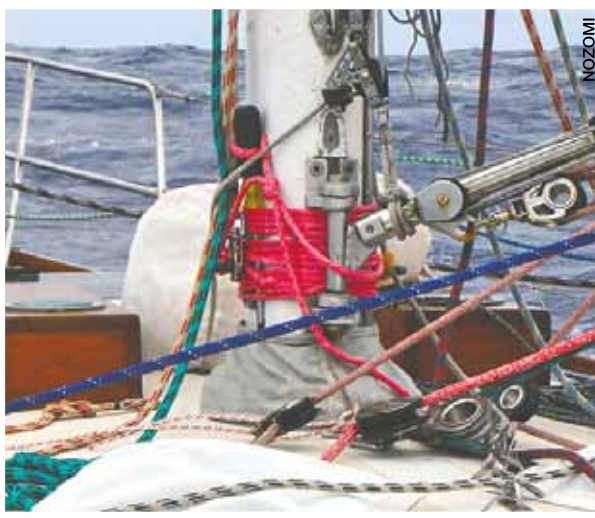
On the doublehanded Cal 40 'Nozomi', Robb Walker secured the vang fitting at the base of the mast with a Spanish windlass.
