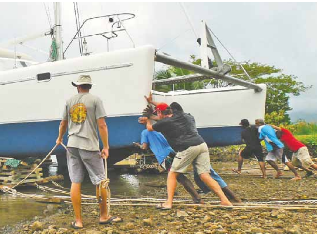
The launch of 'Quixotic'. When you don't have modern equipment and facilities, you simply have to make do with what you've got. In Fiji, that turned out to be a lot of logs from coconut trees and human muscle power. It was a slow but successful process. More next month.
