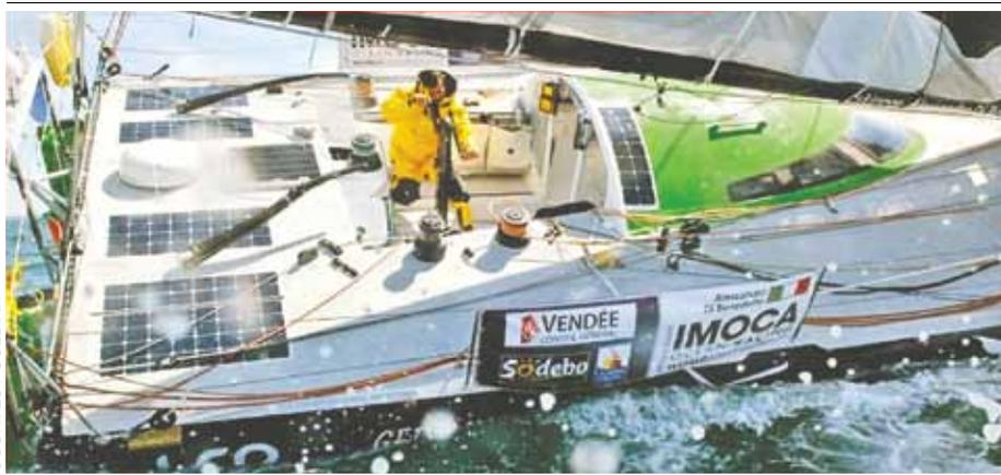
***Around-the-world race boats such as this, need to maximize solar intake in order to keep their high-tech batteries charged.***
