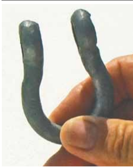
Jim Milski holds up the none-too-robust shackle, minus the crucial pin, that once connected 'Gran Wazoo's' anchor to her rode.
