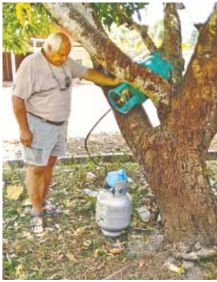
Gene Seybold cools the lower tank when decanting propane by gravity from the upper tank to the lower one. Proper fittings are used.
