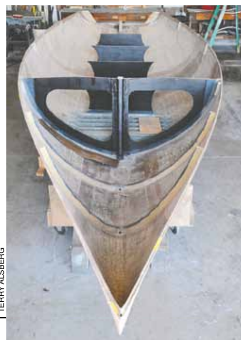
An interior view from before the deck went on. The carbon-fiber bulkheads are nearly weightless, so lightening holes would be overkill.
