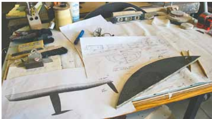
A modern computer rendering rests on the drafting table next to old-fashioned pencil drawings and wafers of bulkhead material.
