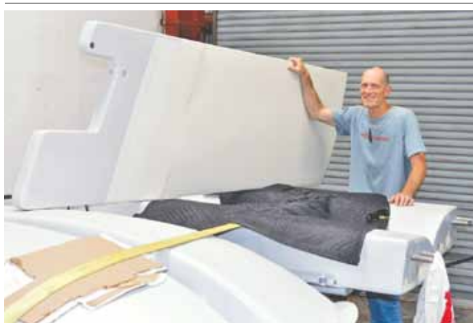
A man and his daggerboard — which will help the tri sail about 40° off the wind. Stacked below it are the ama-attachment beams.
