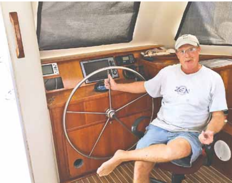
Chris sits at the inside steering position on one of his cats, where it's always dry and shaded. Just to the left is an opening to a 'forward' cockpit, which is great during stints of downwind sailing.
