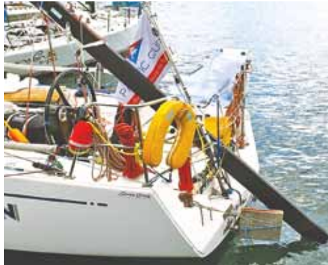
Using the main boom for a rudder on the SC37 'Tiburon' was the 'Manhattan Project' of jury rigs.
