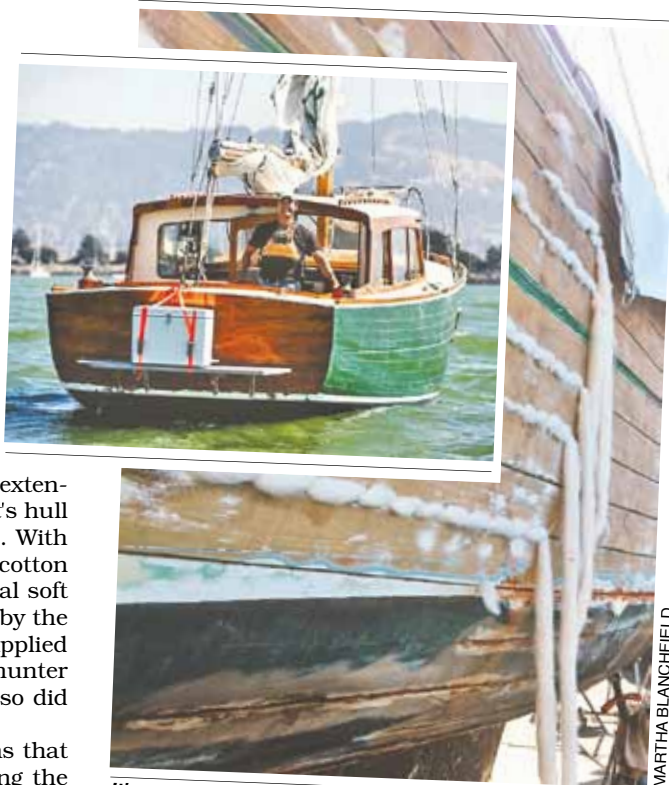
It's not every sailor who knows how to recaulk a seam. Thankfully, that job is now complete.
