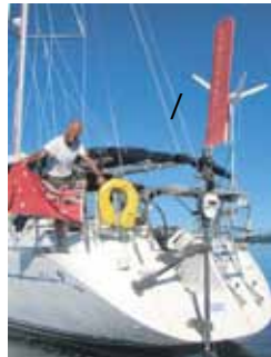
Wayne on SV Dante, his Harmony 42, in Suva, Fiji. Hydrovane mounted off-center to preserve the swim platform.
