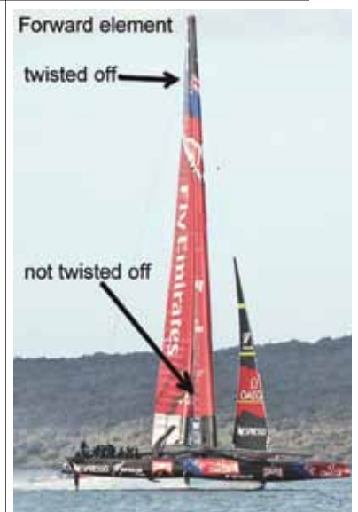
Left: ETNZ's wing has an internal spar covered with a fairing for "leading element twist." Center: OTUSA's wing incorporates the "mast" in a D-shaped leading edge. Look for the "tab" on the trailing edge of the leading element when you get a closeup in the videos." Right: Look closely at ETNZ's wing to see their "leading element twist."
