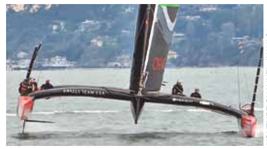
OTUSA's second boat, bow on. In contrast to the Kiwi's boat, it has no diagonal understructure and fine bows.
