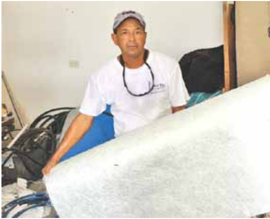
Photos from a refit, clockwise from left. Four 55-gallon drums of epoxy were used. As were a dozen sheets of honeycomb for the new soles. And hundreds of feet of mat and cloth. The new aft cabin hulls feature a thicker inner skin, four additional transverse frames, and four air-tight chambers. Despite all the new weight, 'Profligate' still rides above her lines.
