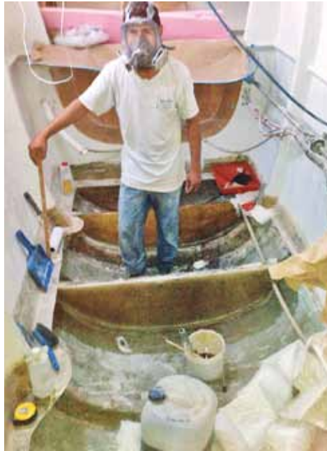
Photos from a refit, clockwise from left. Four 55-gallon drums of epoxy were used. As were a dozen sheets of honeycomb for the new soles. And hundreds of feet of mat and cloth. The new aft cabin hulls feature a thicker inner skin, four additional transverse frames, and four air-tight chambers. Despite all the new weight, 'Profligate' still rides above her lines.
