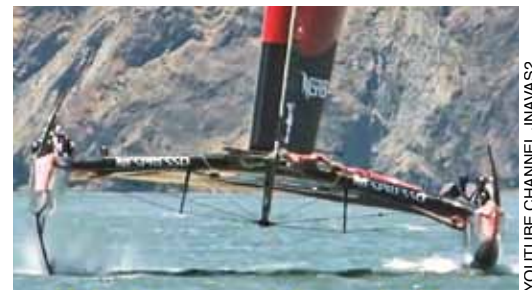
The kiwis sacrificed aerodynamic drag for a stiff platform and high volume bows that have shown their resistance to pitchpoling.
