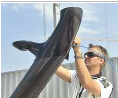
Technician Mark Sheffield adds electronics to the stern post of an AC45. The 72s will carry four cameras, in addition to GPS transponders.
