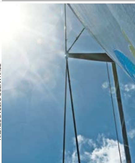
'Team Sanya' fell victim to damage again. This time it was the port D2 shroud that let go. They saved the rig, but had to drop out of Leg Two.
