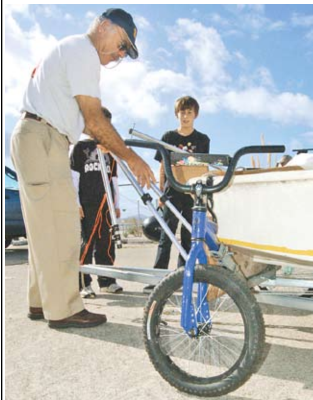
Nice wheels — (clockwise from below) Kame gets his land sailer ready to roll; the front halves of two small bikes act as the boat's rudder; Sam and Kevin show how it's done; wheelchair wheels grace the bow; the whole shebang can fit in the back of a pick-up; Sam, Kame and Kevin didn't want to stop the fun.
