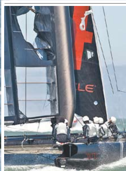
A Coutts-shaped hole in the wingsail was quickly repaired.
