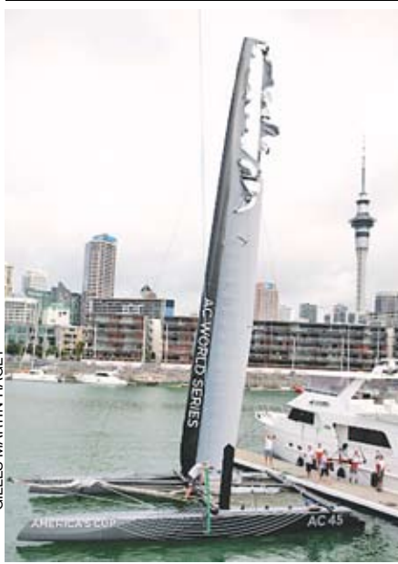
The AC 45 shows off its tattered wing following the capsize. The aft flap is missing, and the skin on the upper portion is shredded to bits.
