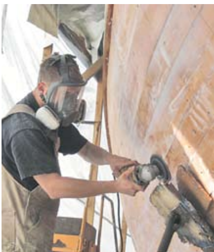
More than 25,000 man-hours have gone into the refit so far. Clockwise from upper left: the look of vertical cold molding; fairing the hull; refurbishing decks; stripping old paint; rebuilding the house; smoothing the final layer of planking.
