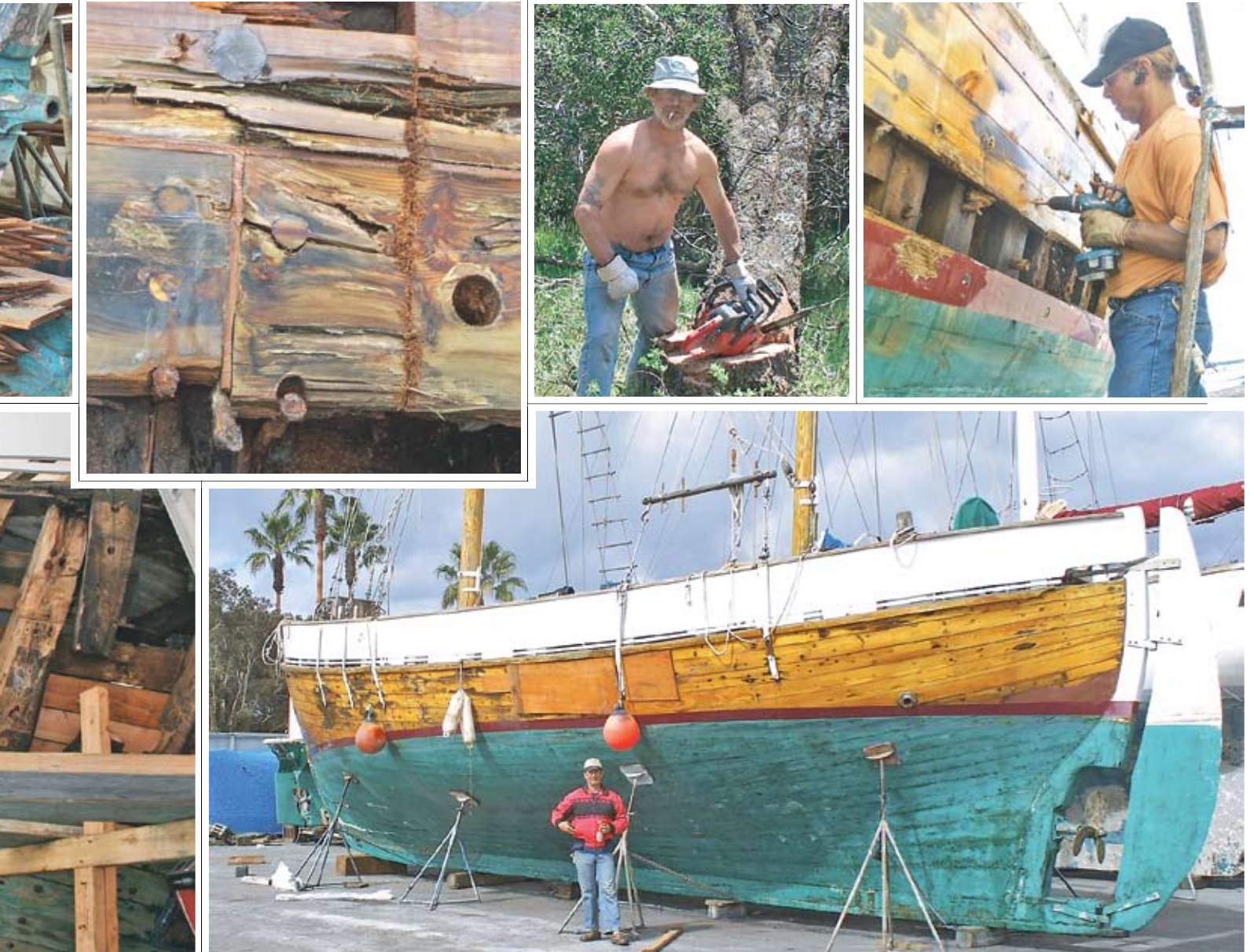
Clockwise from upper left: Repairing damaged ribs; the original planking couldn't be salvaged; cutting oak in the wild for major components; removing damaged planks one by one; safely hauled out after the offshore tow; a view of the original beefy ribs, which were sawn from tree limbs.
