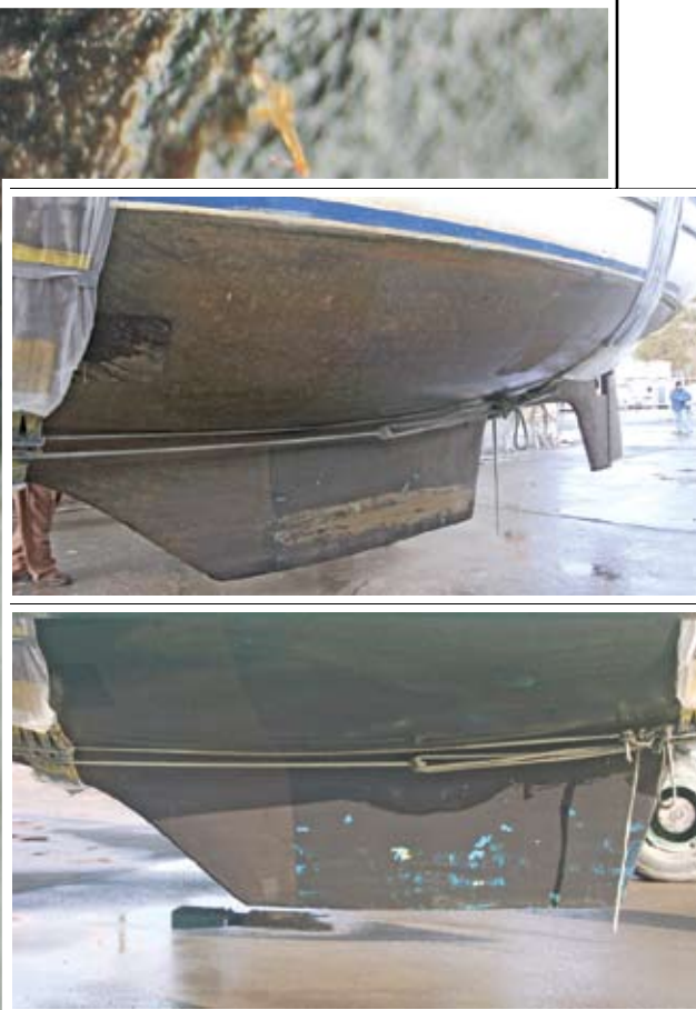
Before and after — the water-based paint (right) is still performing noticeably better than the other paints but doesn't seem to stand up to pressure washing as well as the other paints — though Jack Hickey says it's actually much harder.
