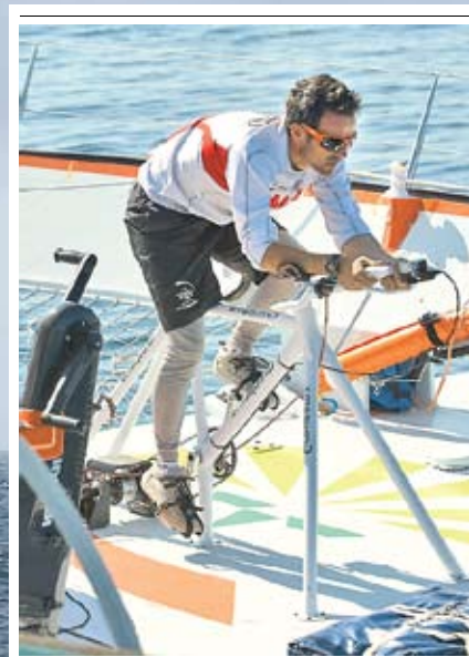
Spread, Franck Cammas will be sailing his 105-ft tri 'Groupama 3' in the Route du Rhum. Inset, Cammas can grind winches via a custom-designed bicycle-style pedestal.
