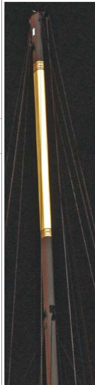
Reflective personality — Clockwise from below, 3M Scotchlite 680, seen here glowing in the sun, is much easier to handle when cut into smaller pieces; an epoxy scraper works perfectly to smooth out wrinkles and bubbles; we used thin strips to 'finish' the vinyl job and added SOLAS-approved white reflective stickers at the top of the mast; at night, our mast really shines; Spaulding Center boatyard manager Michael Wiener was really impressed with our handiwork. "Your mast is beautiful," he said. We think so too!
