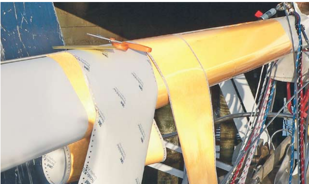
Reflective personality — Clockwise from below, 3M Scotchlite 680, seen here glowing in the sun, is much easier to handle when cut into smaller pieces; an epoxy scraper works perfectly to smooth out wrinkles and bubbles; we used thin strips to 'finish' the vinyl job and added SOLAS-approved white reflective stickers at the top of the mast; at night, our mast really shines; Spaulding Center boatyard manager Michael Wiener was really impressed with our handiwork. "Your mast is beautiful," he said. We think so too!
