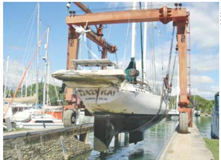
The big Long Beach-based schooner 'Cocokai' being lifted out of the water in Fiji for a major haulout. The price was right.
