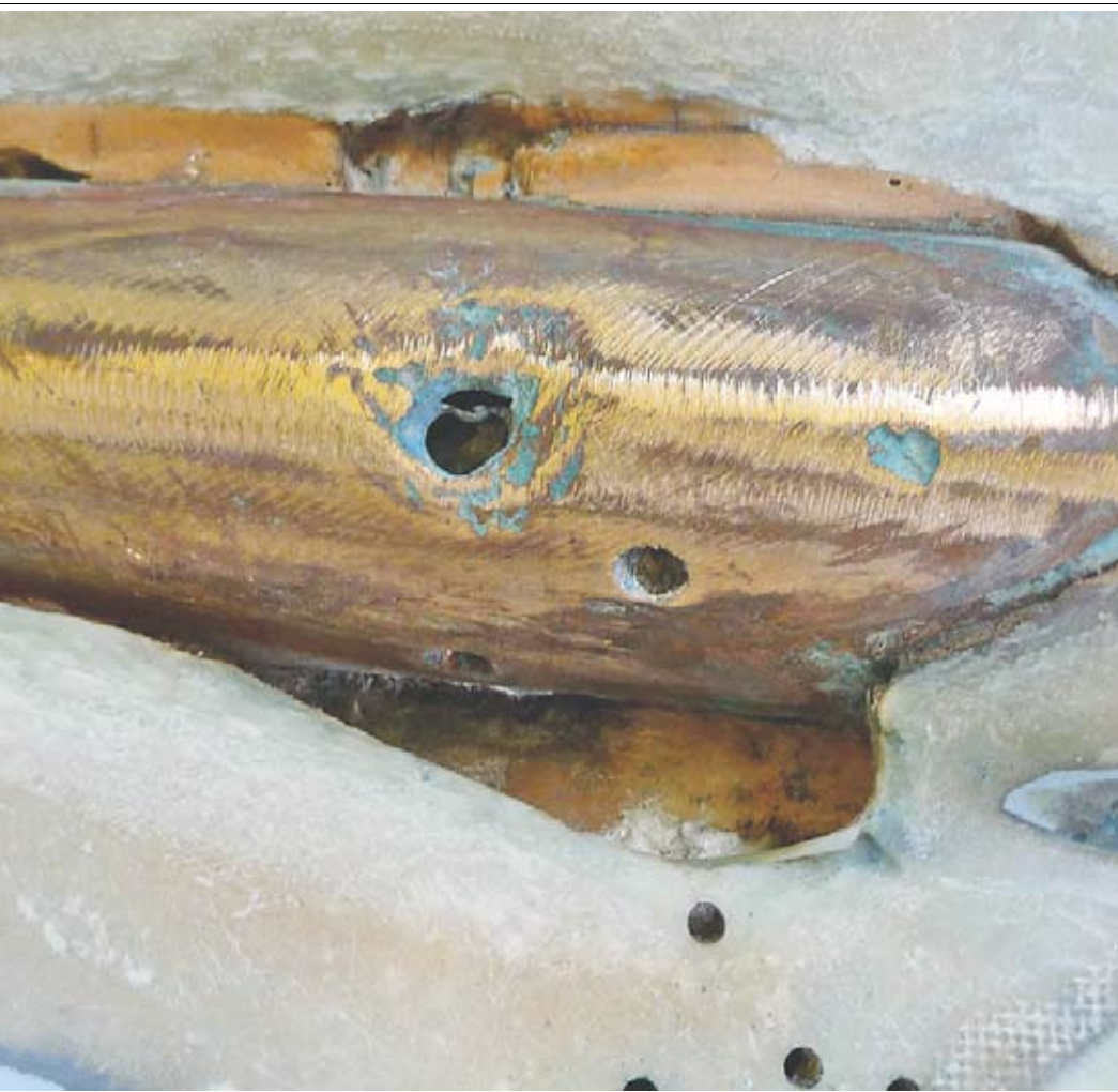
The shaft tube on 'Swell', complete with holes in the tube and the surrounding layout. The hope was that glassing it all up would stop the leak.
