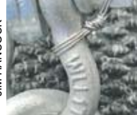
A proper 'mousing' job on a shackle.
